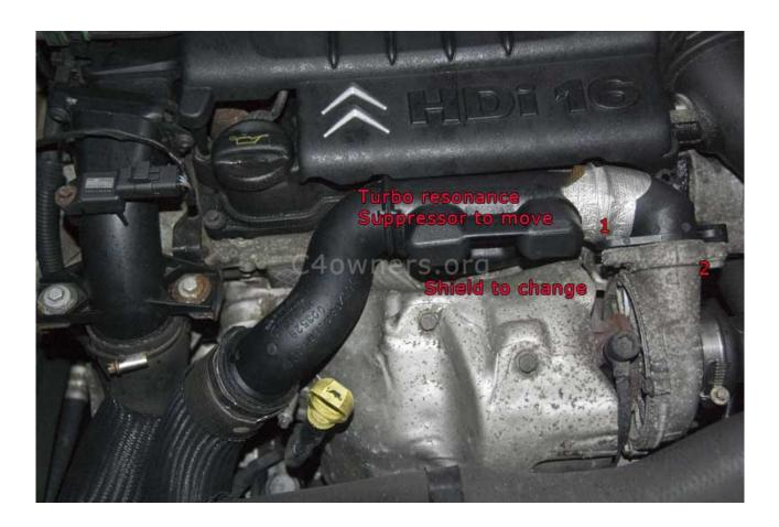
Step one is to remove the Engine Cover and Turbo Resonance Suppressor to gain access to the engine side securing bolts. For this you only need a 10mm combination spanner (open jaw and ring) as there is no room for a socket.
