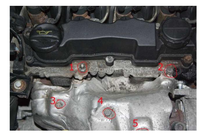
Now you need to remove the 5 bolts indicated to free the broken part of the heat shield.
